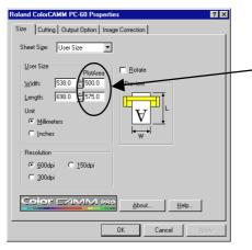
We will devide the data in half so we will set the [Length] to the half of the size of the current size and press OK button.
